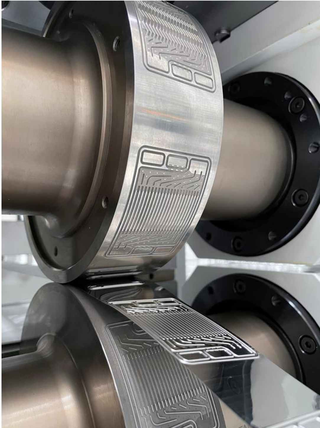
Roll embossing of bipolar plates using BPPflexRoll. © Fraunhofer IWU
