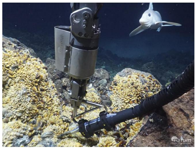
In the field studies on black smokers, robots are used to depths as great as 3000 meters; they are equipped with extensive sensor technology and can take samples of the fluids and rocks. MARUM
