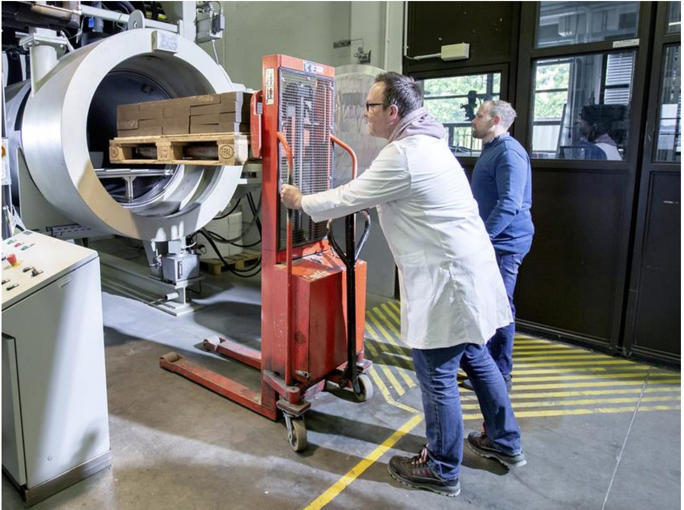
Michael Prokein (left) and Jannick Armenat from Ruhrstoffbauwerke at the pre-industrial plant for hardening building materials and CO 2 storage. Fraunhofer UMSICHT
