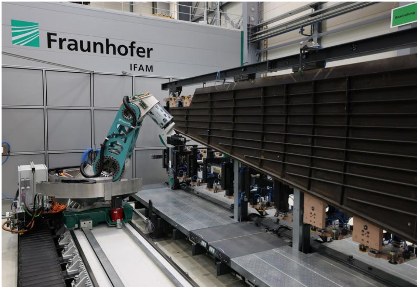
The newly developed flexible milling kinematics with hybrid drive on a linear axis machines a CFRP vertical tail plane of an aircraft on a 1:1 scale with high precision © Fraunhofer IFAM
