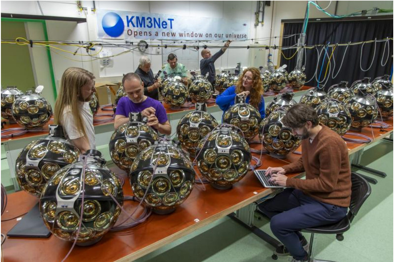
An assembly of digital optical modules which later become a part of the KM3NeT neutrino telescope in the Mediterranean Sea. The KM3NeT Collaboration
