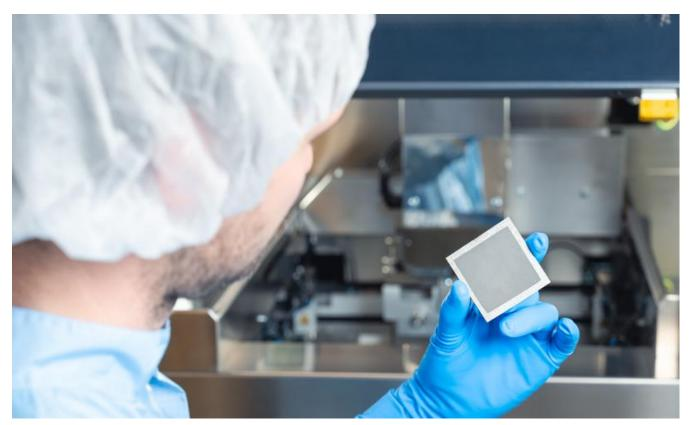
Final microporous layer on a titanium fibre substrate after the screen printing process. In a subsequent step, the two layers are sintered. The microporous layer with a reduced surface roughness allows an optimized interface to the catalyst layer.
