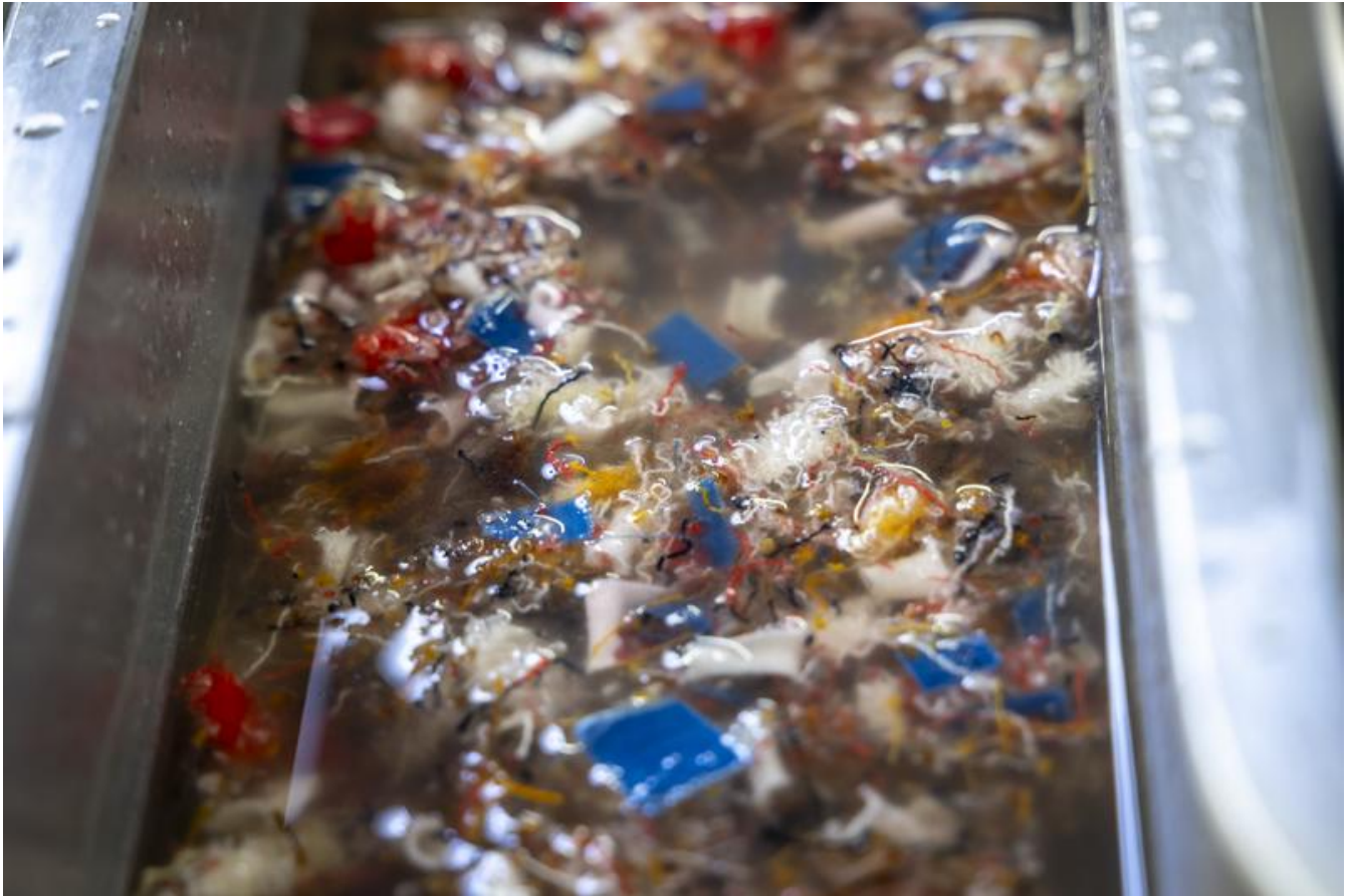
To make paper from old items of clothing, they are first cut into small shreds and soaked in an aqueous solution. Helmut Lunghammer Lunghammer - TU Graz
